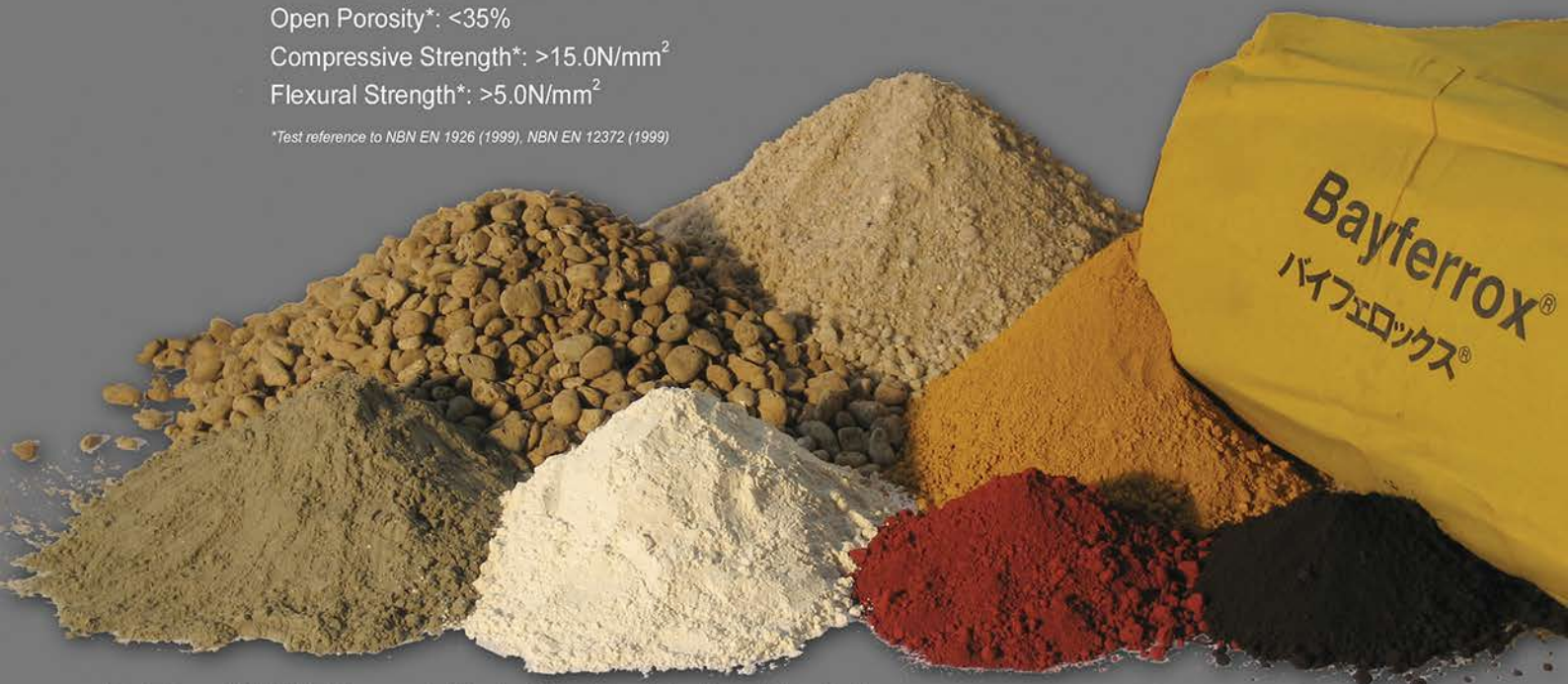
Back Row: Light-Weight Aggregate (Pumice Stone), Sand, BayFerrox's Iron Oxide. Front Row: Portland Cement, White Cement, BayFerrox's Iron Oxide.
